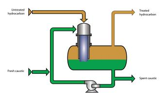
NAPFINING™ and NAPFINING™ HiTAN technologies employ the FIBER FILM® Contactor as the mass transfer device and utilize caustic as the treating reagent to remove naphthenic acid compounds mainly from jet fuel, kerosene, diesel, condensate and crude oil streams.
