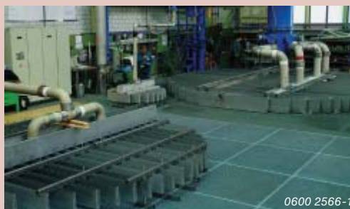
Liquid distributor test to confirm the correct operation range of each distributor
