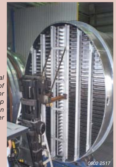
Vibration test, to simulate transportation of assembled columns / cold boxes
