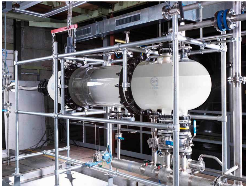
Fig. 18a: Test rig for Sulzer Mellaplate and DC Coalescer
