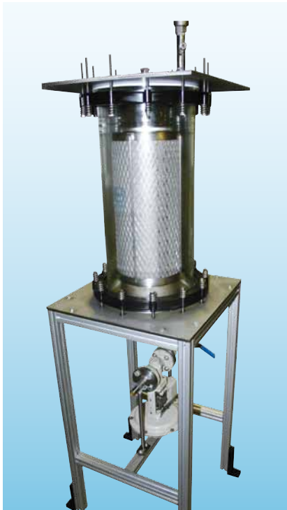
Fig. 18b: Sulzer Dusec test rig for customer tests on site
