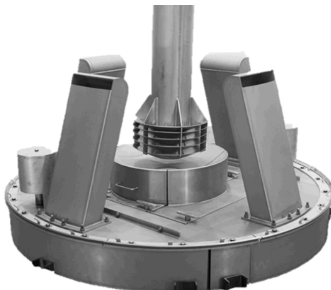
The design of the gas phase scale catcher ensures that fines, scales, corrosion products and inorganic matter in the gas are removed. During turnaround the scale catcher can easily be accessed from the top of the reactor for cleaning.
