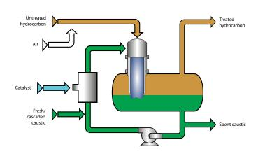
MERICAT™ technologies employ the FIBER FILM® Contactor as the mass transfer device and utilize a caustic/catalyst/air mixture as the treating reagent to remove hydrogen sulfide and sweeten mercaptan compounds in gasoline/naphtha, condensate and crude oil streams.
