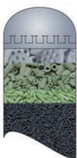
Figure 3: Typical example of Topsøe graded bed solution.
