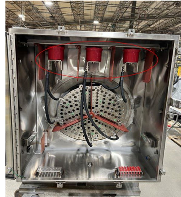
~1 MW medium Voltage Heater (4160V)
