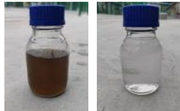
Comparison of water inlet and outlet of the unit
