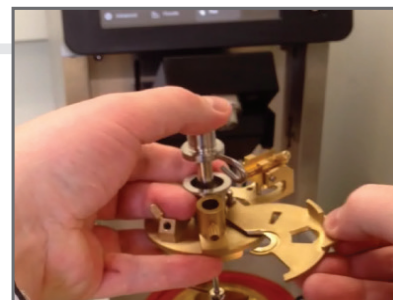
Easy disconnection, for easy and external cleaning of the cup-cover
