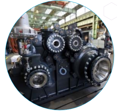
CO 2 (8 stage) "Urea" Delivery 2015, in operation
