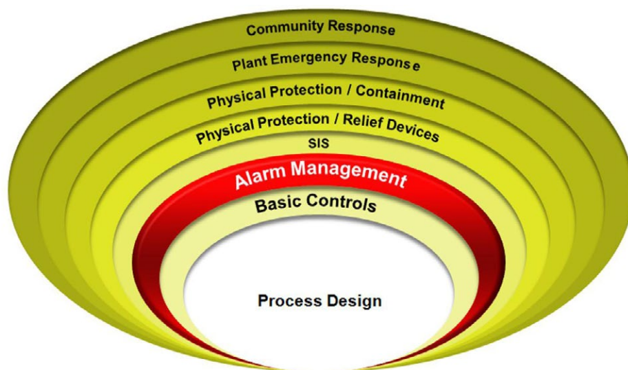
Figure 1: Layers of Protection in a Processing Plant
