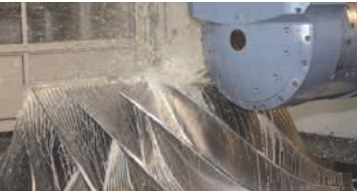
Inside the 5-axis machine: the milling process
