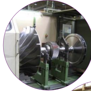
Low and high-speed balancing of rotors
