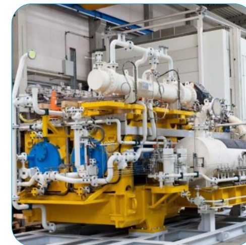
Instrument Air Compressors
