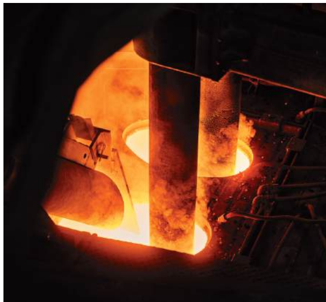
Figure 1 Pyro-metallurgical processes are required to recover and refine every possible ounce of precious metals like rhenium (Re) from catalytic operations in refinery and petrochemical facilities
