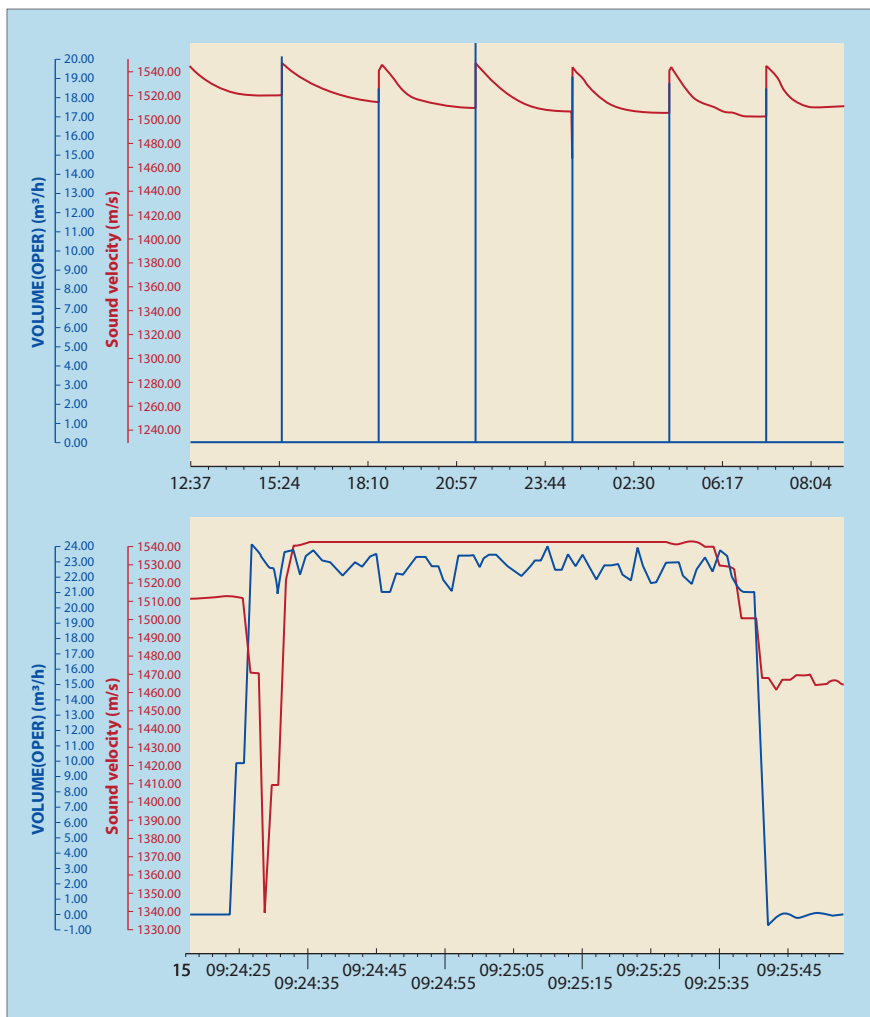
Figure 3 Sound velocity dewatering system – draining cycle operation (blue line is flow measurement, red line is sound velocity measurement)
