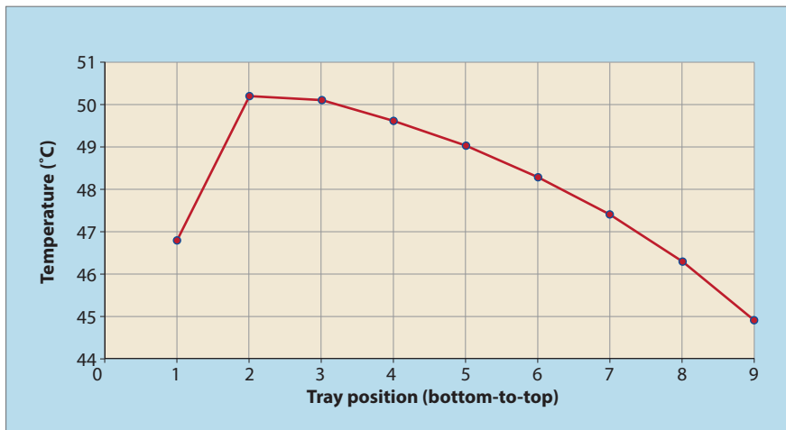
Figure 10 Stage-wise (bottom-to-top) temperature profile (conversion = 30 %, feed S = 1.7%, amine flow = 80 t/h)
