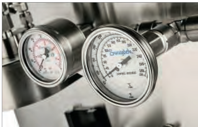
Figure 2 Installing a pressure gauge before and after a control valve and on a condensate return leg after the steam trap helps to provide accurate data for monitoring a steam system
